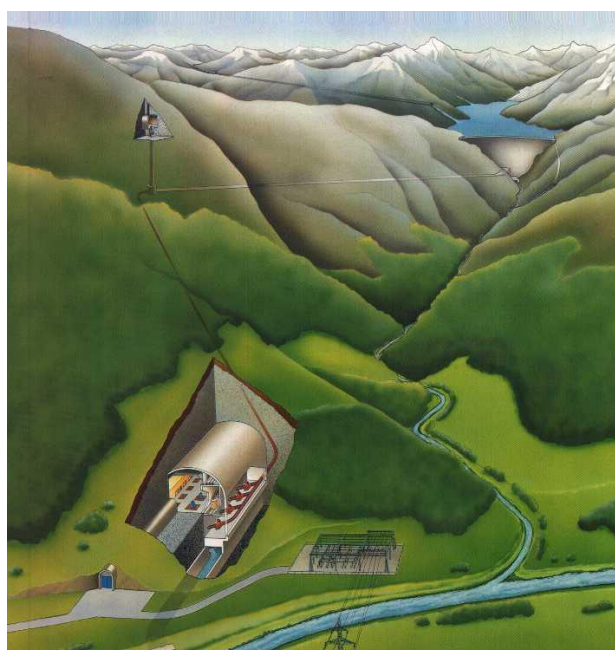
Figure 2-2 – Overview of a storage hydropower plant with main elements starting from reservoir fed eventually by diversion tunnels from neighbouring catchment, arch dam, power intake, pressure tunnel, surge tank, pressure shaft, underground powerhouse, tailrace channel and switchyard.
