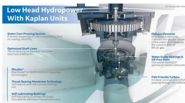
Figure 5-9 – Kaplan turbine (source: GE)
