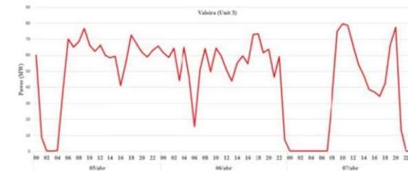
Figure 4: Typical operation scheme of Valeira over 3 days
